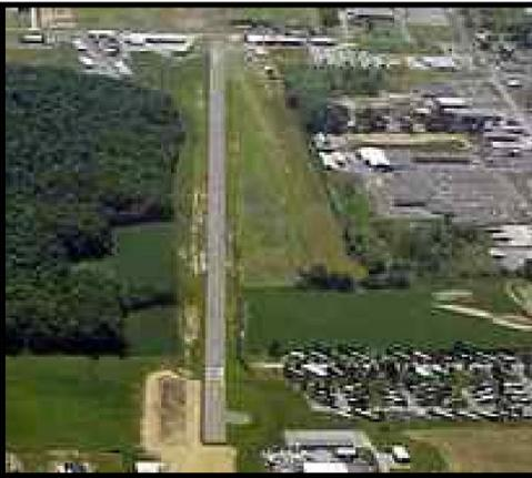
The Willard Airport is open to the public and is located just south of and parallel to the commercial corridor located along U.S. Route 224. The runway measures 4,028 by 65 feet, and the surface is asphalt in good condition. There are medium intensity edge lights. Fuel is available on site, provided by Willard Aviation.
